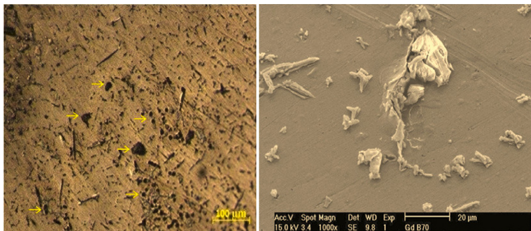
Fig. 2. Metallographic (left) and SEM (right) pictures showing the bigger hydride precipitates above which the oxide layer has been ruptured. These are the initial development centers of the so-called “growth centers” (GCs). The main GCs on the metallographic picture are indicated by arrows.
